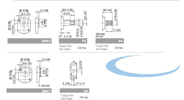
Maximum torque ratings are referred to ideal working conditions; such values may reduce based on the quality of joints and connections used..
